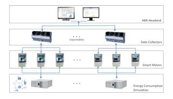
A further extension of SecLabE with an AMI is planned. The structure of the AMI is presented in the following diagram where hardware components such as smart meters and data collectors will be directly connected to a simulation of the energy consumption.
