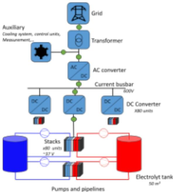
Plan of the entire Redox-Flow-Storage system. From bottom to top: The tank, the pump system and the stacks from which DC voltage is stepped up to approx. 600 V. The current is collected on the high-voltage bus and converted into AC in order to feed it into the grid. The green dots mark the measuring points for operational analysis and efficiency calculation.
