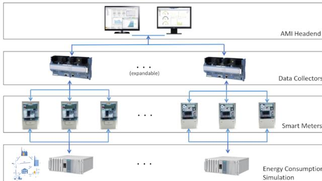
A further extension of SecLabE with an AMI is planned. The structure of the AMI is presented in the following diagram where hardware components such as smart meters and data collectors will be directly connected to a simulation of the energy consumption.
